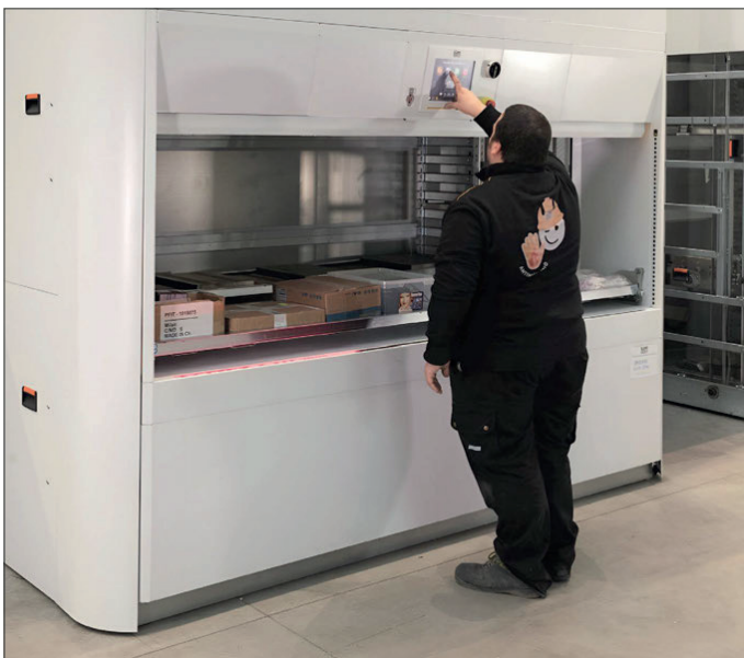
With a Modula VLN, goods are brought directly to the picker
